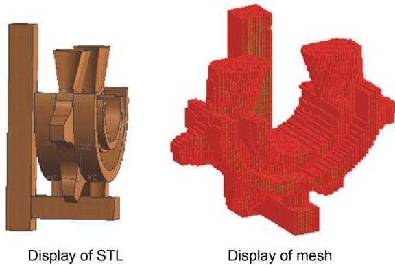
Fig. 3: Chain-wheel mesh generation
