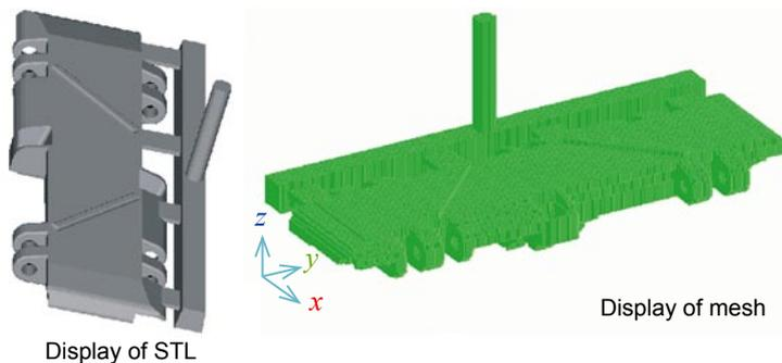
Fig. 4: Creeper tread mesh generation
