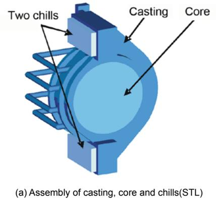
(a) Assembly of casting, core and chills(STL)
