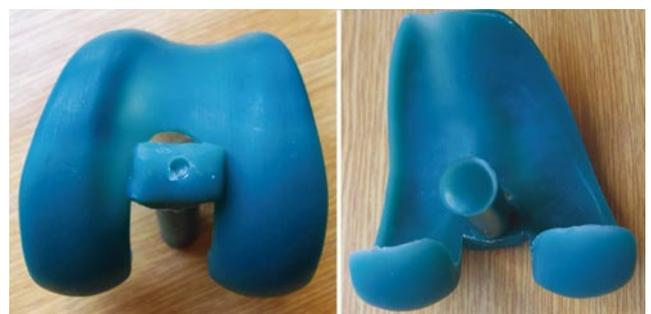
Fig. 8: Prototype of wax pattern for investment casting technology
