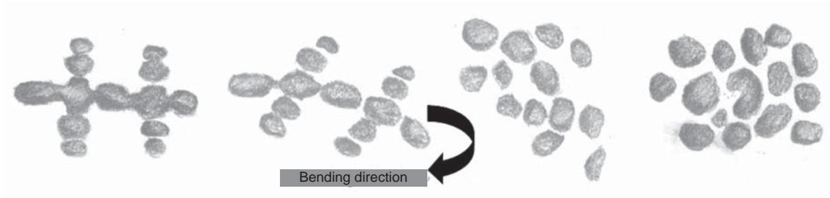
**Fig.4: Schematic illustration of microstructural evolution of white cast ingots agitated by electromagnetic field during isothermal stirring**
