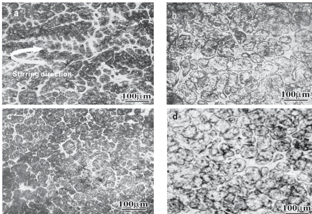
**Fig.3: Evolution of microstructure morphologies in white cast iron ingots solidified after stirring for 5 s (a), 15 s (b), 120 s (c) and 240 s (d)**
