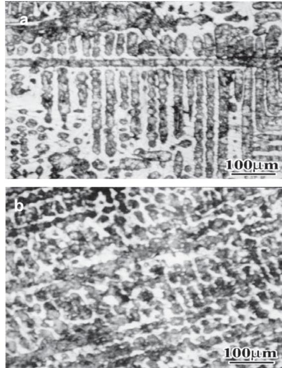
**Fig.2: Microstructures taken from (a) boundary and (b) internal of white as-cast iron ingots**
