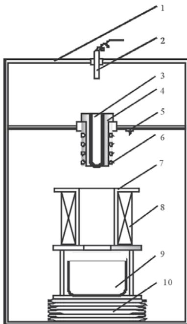
1. Chamber; 2. Radiation pyrometer; 3. Quartz crucible; 4. Graphite crucible; 5. Touching switch; 6. Induction coils; 7. Water cooler; 8. Electromagnetic stirrer; 9. Melt collector or quenching basin; 10. Elevating mechanism
