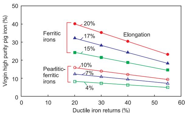
Fig. 3: HPPI – DIR relationships for different elongation levels in ductile irons (DI)
