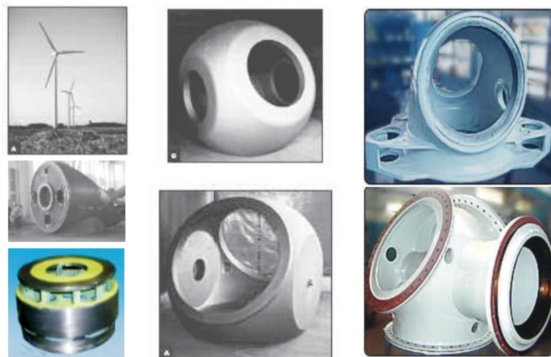
Fig. 1: Typical ductile Iron (DI) castings for windmills
