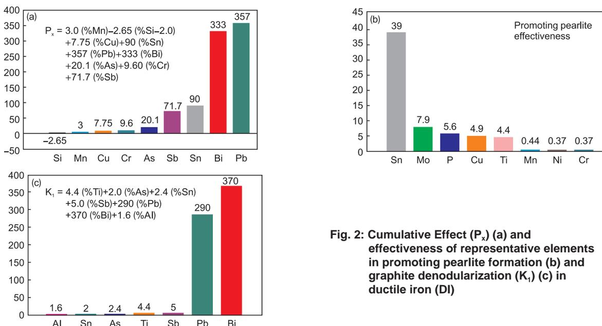
Fig. 2: Cumulative Effect ( $P_x$ ) (a) and effectiveness of representative elements in promoting pearlite formation (b) and graphite denodularization ( $K_1$ ) (c) in ductile iron (DI)
