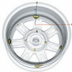
Fig. 13 Predicted shrinkage defects under forced-cooling
