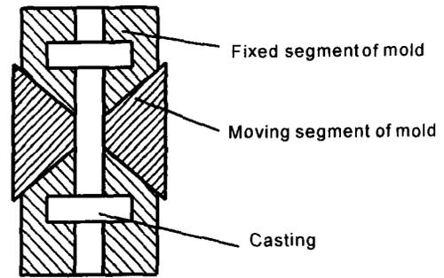
Fig.1 Sketch map of the shape of guide vane casting and mold with yieldability.
