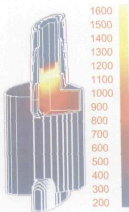
Fig.2 The temperature field at 15 860 s for ESRC guide vane casting
