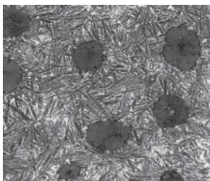
Fig. 3 Typical microstructure of ADI grade 1
