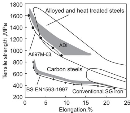
**Fig.2 Comparison of ADI properties with steels and conventional ductile irons; ADI standard A897 M-03 and BS EN 1563-1997 also shown in figure**
