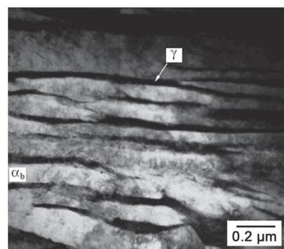
Fig. 4 TEM ADI microstructure showing ferrite plates in acicular structure, separated by thin films of austenite [4]
