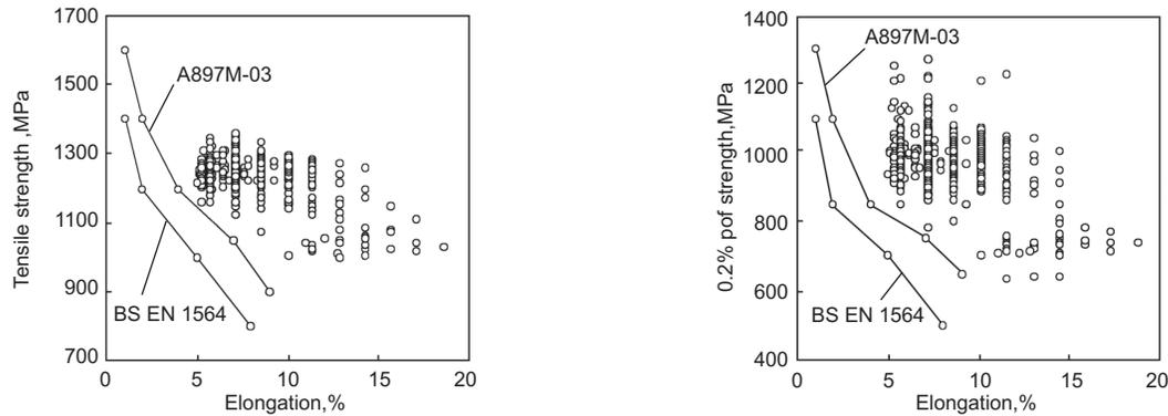
**Fig. 5 ADI tensile strength vs elongation (left) and 0.2% proof strength vs elongation (right)**
