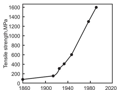
Fig.1 The increase of cast iron strength with year
