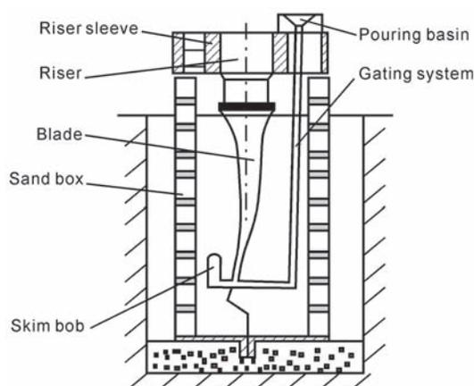
Fig. 1 process drawing for hydroturbine blade casting
