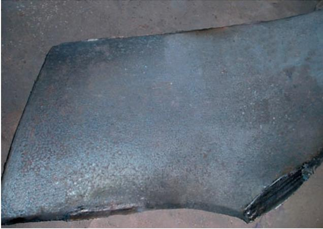
**Fig. 5 Trial blade casting free of surface defects**
