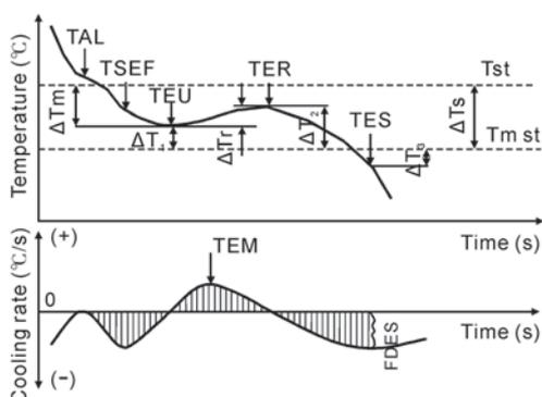
Fig. 1 Typical cooling curve and its first derivative of hypoeutectic grey cast iron
