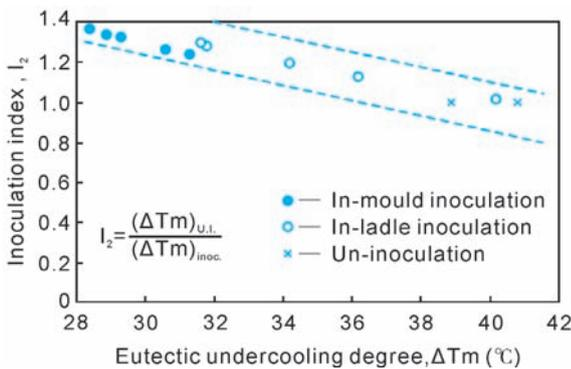
Fig. 4 Inoculation Index ( $I_2$ ) of treated irons
