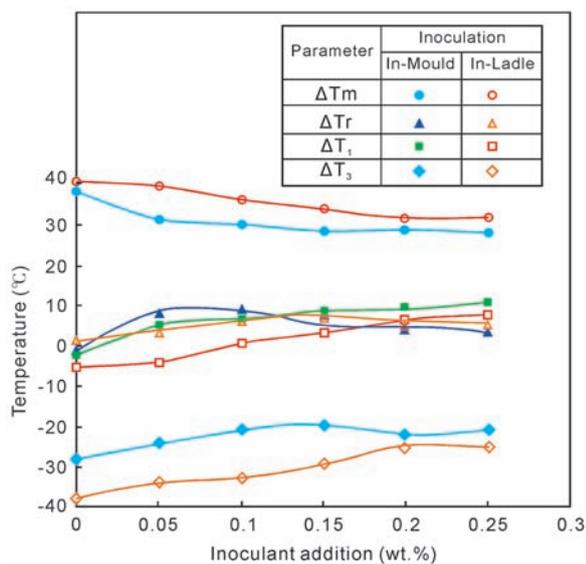
Fig. 2 The influence of the inoculant addition amount and inoculation method on the representative thermal analysis parameters
