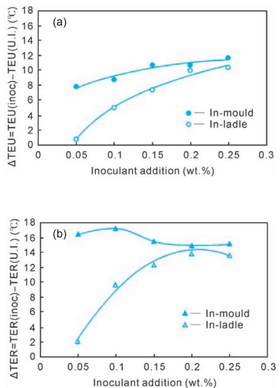
Fig. 3 Undercooling (a) and recalescence (b) difference between un-inoculated and in-mould/in-ladle inoculated irons
