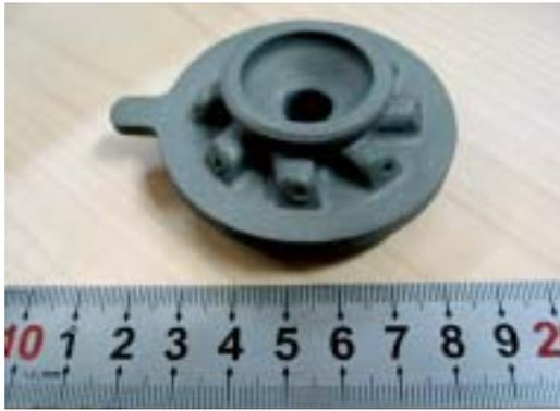
Fig. 3 TiAl vortex agitator casting
