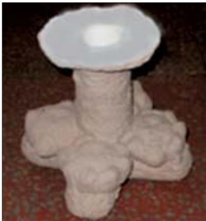
Fig. 1 The baked oxide ceramic shell
