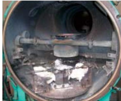
Fig.2 The melting and centrifugal casting furnace
