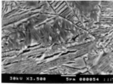
Fig. 3 Martensite formed in austenite zones between ausferrite platelets in 2%Ni alloyed ADI, ausformed to 25% reduction and austempered at 375°C for 1 min
