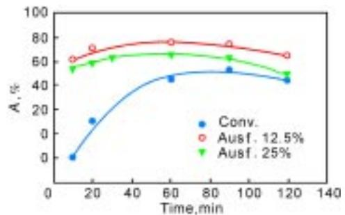
Fig. 7 Total elongation vs austempering time and ausforming reduction for ADI alloyed with 2% Ni
