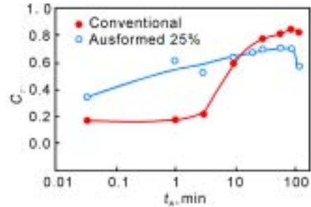
Fig. 5 Variation of total carbon content of saturated austenite  $C_{\gamma}$  with austempering time for conventional and ausformed to 25% ADI alloyed with 2% Ni
