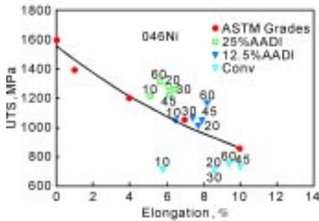
**Fig. 8** Ultimate tensile strength versus ductility for 12.5% and 25% ausformed and conventionally austempered specimens along with ASTM minimum requirements for ADI. The austempering time specified (in min) adjacent of the point
