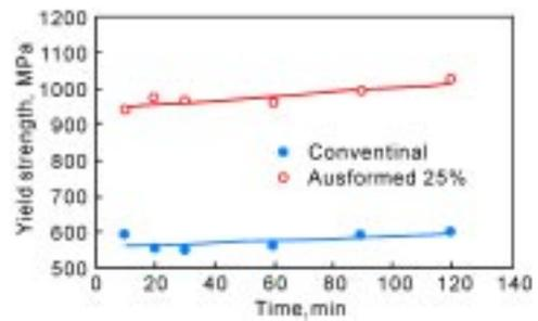
Fig. 6 Yield strength vs austempering time and ausforming reduction for ADIs alloyed with 2% Ni
