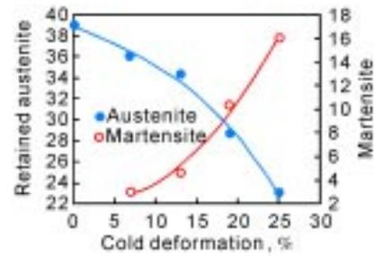
**Fig. 10** Variation of volume fractions of retained austenite and mechanically formed martensite with cold reduction pct
