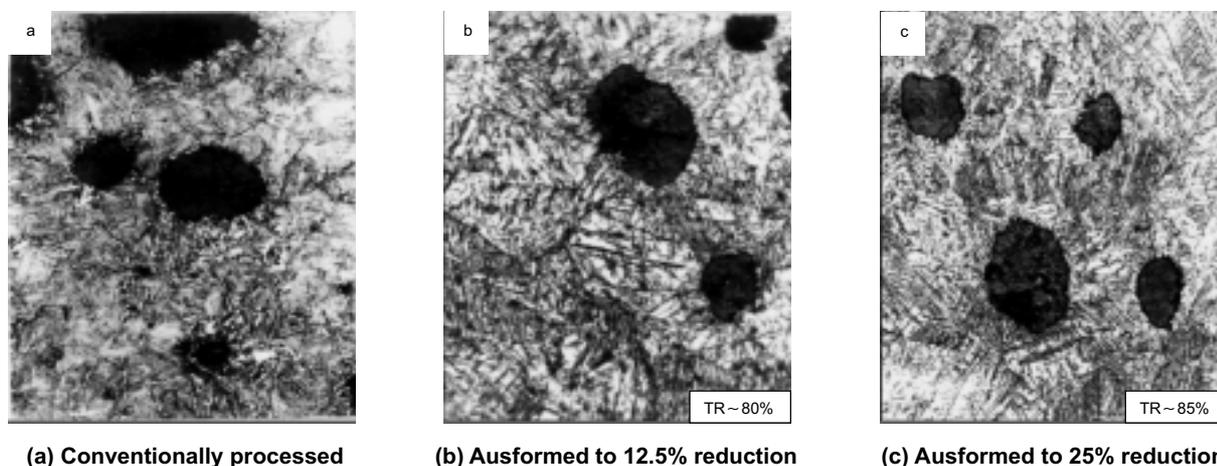
**Fig. 1 Photomicrographs of ADI alloyed with 2%Ni austempered at 375°C for 10 minutes after different ausforming reductions**
