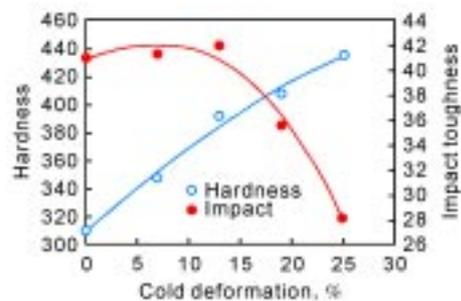
**Fig. 13** Variation of Vickers hardness and impact toughness with cold reduction pct
