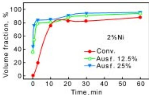
Fig. 4 Volume fraction of transformation versus austempering time for 2% Ni alloyed ADI
