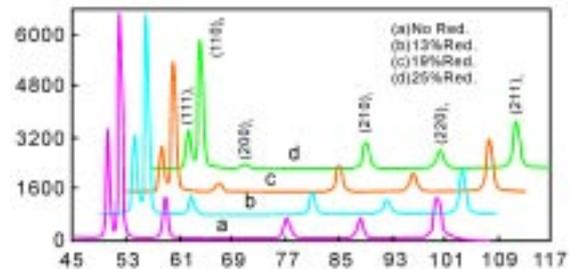
**Fig. 11** Variation of peak intensity for  $\gamma$ - and  $\alpha+\alpha'$  phases in unalloyed ADI
