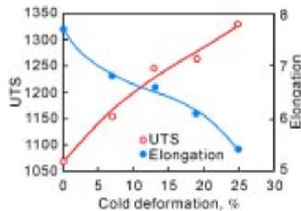
**Fig. 12** Variation of elongation and ultimate tensile strength with cold reduction pct
