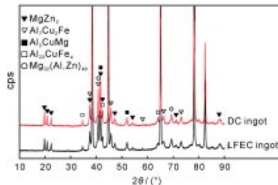
**Fig.3 XRD graph of LFEC and DC ingots**
