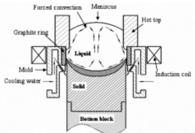
Fig.1 Schematic diagram of LFEC process
