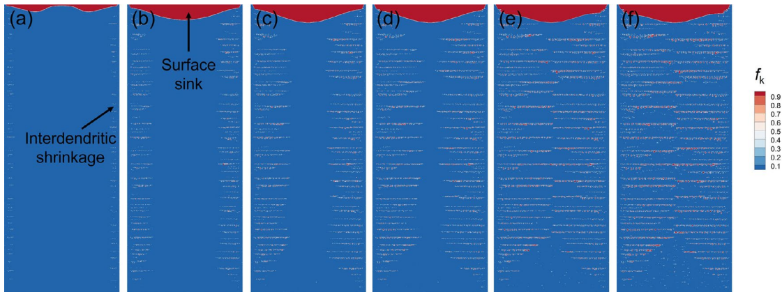
Fig. 12: Shrinkage field evolution for Al-4.7wt.%Cu ingot: (a) 2 s; (b) 7 s; (c) 15 s; (d) 30 s; (e) 50 s; (f) 110 s
