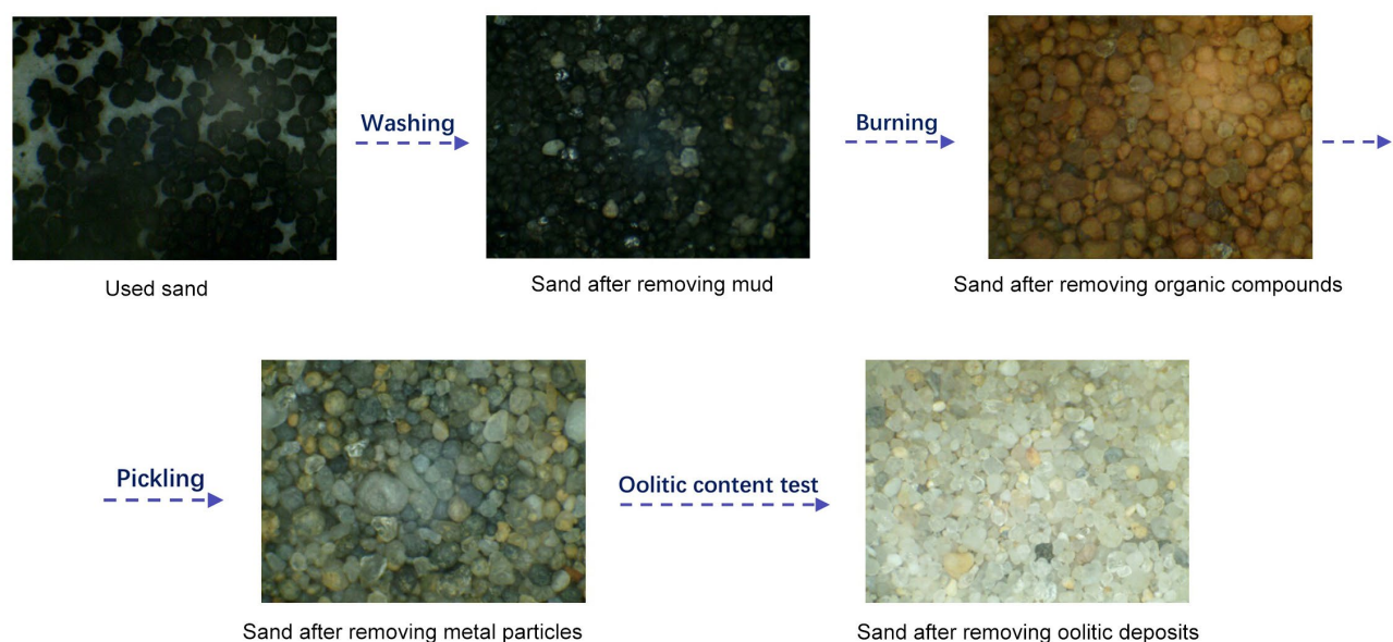
Fig. 1: Pretreatment steps and changes in sands morphology
