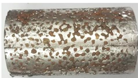
Fig. 2: ASF sample with PEC filler particles
