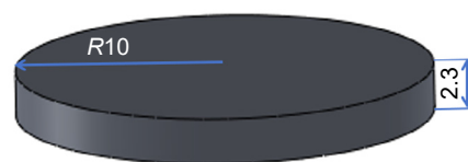
Fig. 2: Geometry and sizes of conductive sample (units: mm)
