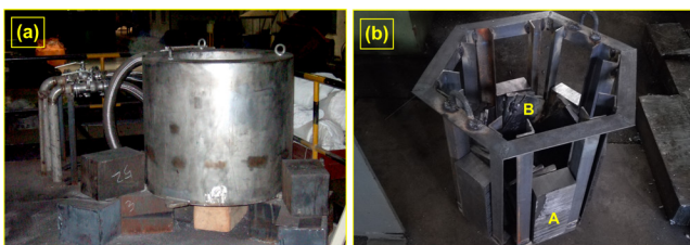
Fig. 2: Single winding helical electromagnetic stirring apparatus (a) and internal magnetic yoke structure (b); A-Yoke back, B-Inclined yoke to generate helical electromagnetic force
