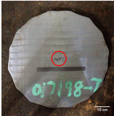
Fig. 3: Star shaped defects in center of ingot cross section
