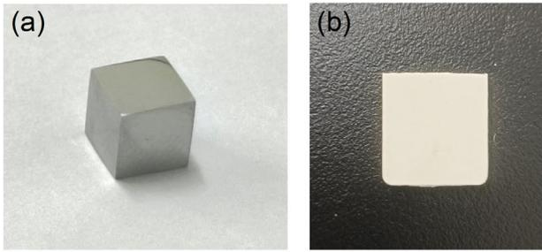
Fig. 1: Sessile-drop experiment samples: (a) 4777DS1 alloy; (b) ceramic core
