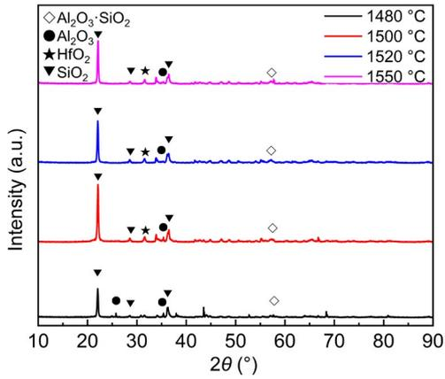
**Fig. 9: Phase analysis of the surface of ceramic cores at different temperatures**
