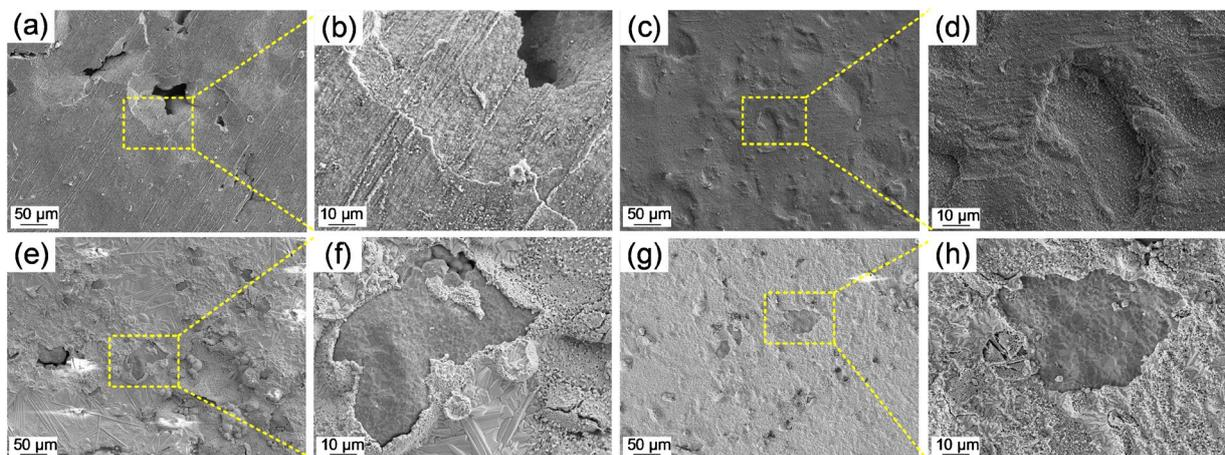
Fig. 5: Microscopic morphology of the bottom surface of 4777DS1 alloy drops after sessile-drop experiments: (a) and (b) 1,480 °C; (c) and (d) 1,500 °C; (e) and (f) 1,520 °C; (g) and (h) 1,550 °C
