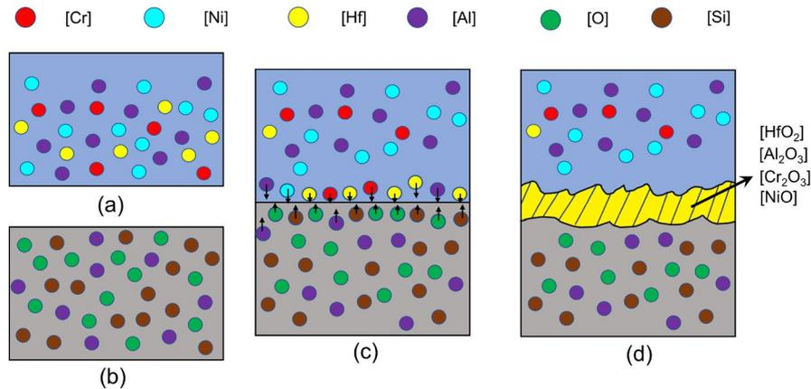
**Fig. 12: Schematic illustration of interfacial reaction processes between 4777DS1 alloy and ceramic core: (a) atoms produced by dissolution of superalloy; (b) atoms produced by decomposition of ceramic core; (c) diffusion of active atoms from alloy matrix and ceramic core to alloy/ceramic interface; (d) reaction products formation by substitution reaction<sup>[27]</sup>**
