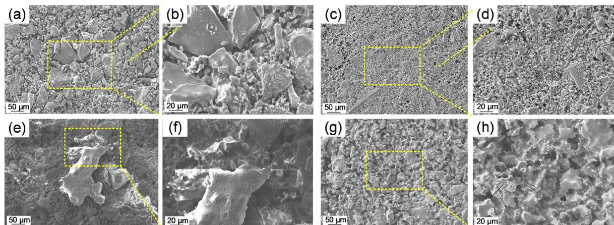
Fig. 8: Microscopic morphology of surface of ceramic core after sessile-drop experiments: (a) and (b) 1,480 °C; (c) and (d) 1,500 °C; (e) and (f) 1,520 °C; (g) and (h) 1,550 °C
