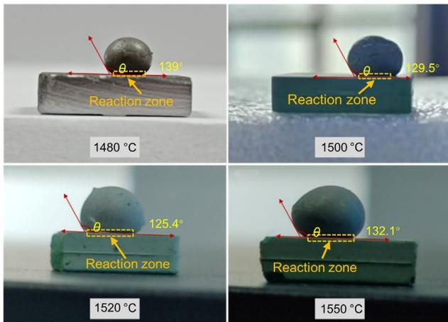
Fig. 4: Macro photographs of wettability angles between 4777DS1 alloy melt and ceramic core substrate at different temperatures
