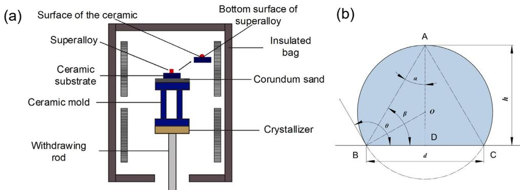
Fig. 3: Schematic diagram of the sessile-drop experiment (a) and measurement method for alloy-ceramic wetting angles (b)
