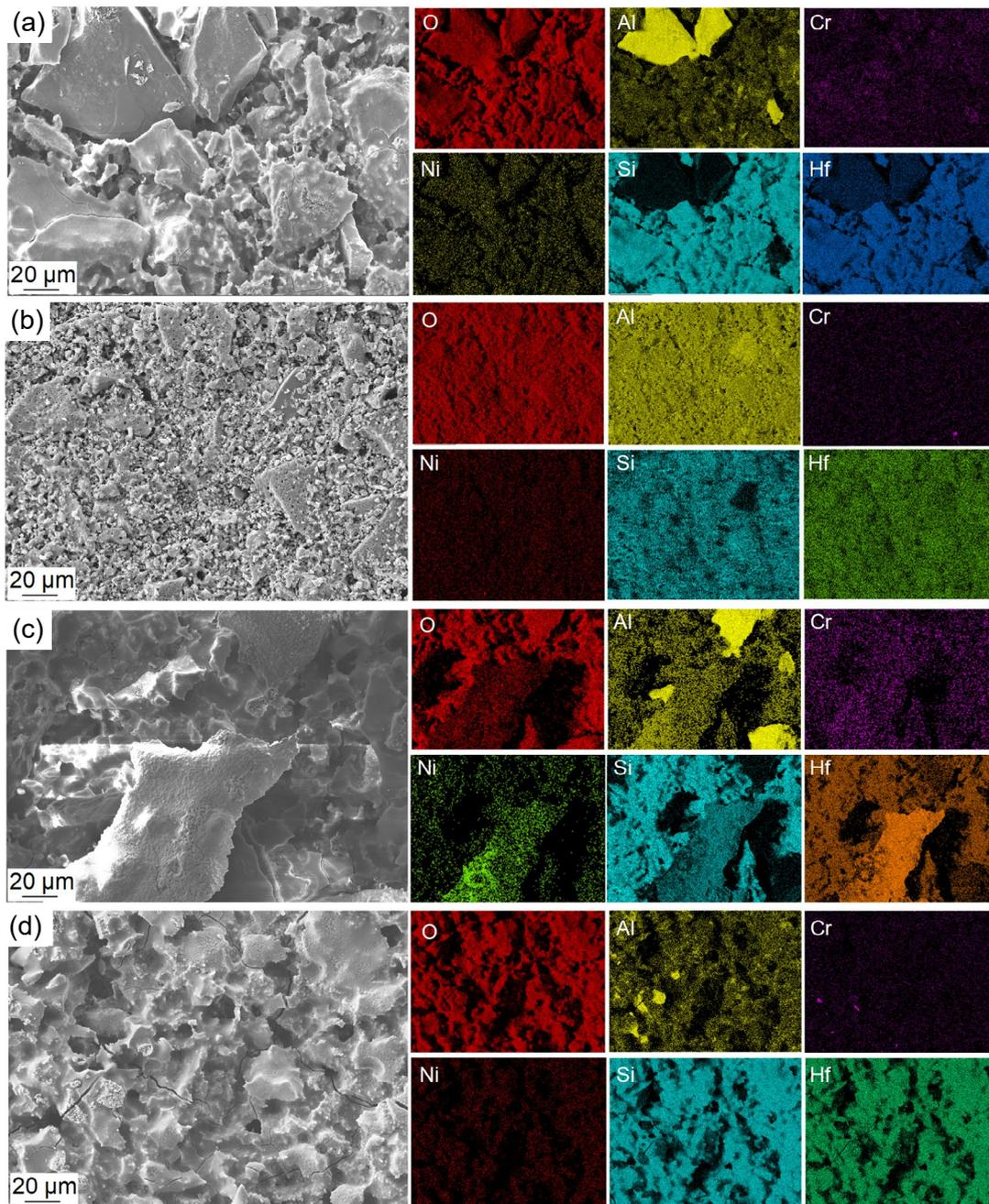
**Fig. 10: Microstructure and element distribution of the surface of ceramic cores at different temperatures: (a) 1,480 °C; (b) 1,500 °C; (c) 1,520 °C; (d) 1,550 °C**
