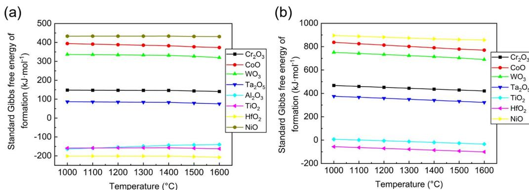
Fig. 11: Standard Gibbs free energy of possible reaction between main elements of 4777DS1 superalloy and ceramic core at temperatures ranging from 1,000 °C to 1,600 °C: (a) SiO<sub>2</sub>; (b) Al<sub>2</sub>O<sub>3</sub>
