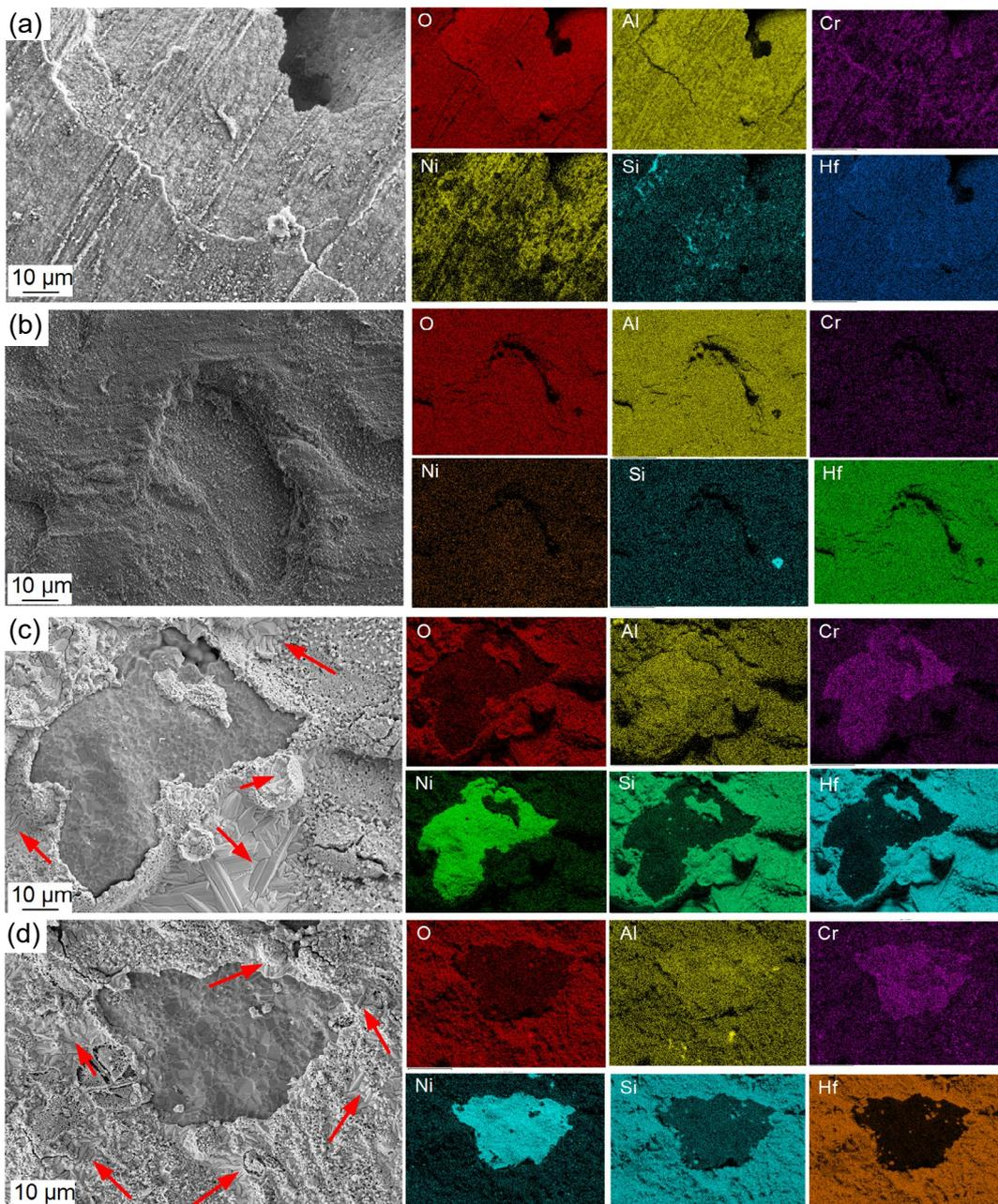
**Fig. 7: Microstructure and element distribution of bottom surface of 4774DS1 alloy drops at different temperatures: (a) 1,480 °C; (b) 1,500 °C; (c) 1,520 °C; (d) 1,550 °C**
