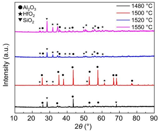
**Fig. 6: Phase analysis of bottom surface of 4774DS1 alloy drops at different temperatures**
