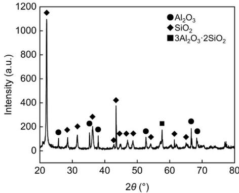
Fig. 2: Phase analysis of the surface of ceramic core before sessile-drop experiment
