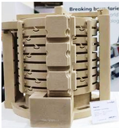
Fig. 11: 3D printing with cold-curing inorganic binders [44]
