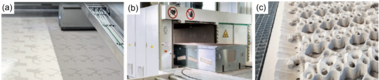
Fig. 10: Pictures of inorganic binder 3D printing (a), microwave curing (b), and sand core samples (c) [43]
