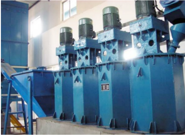
Fig. 18: Multi-barrel strong scrubbing wet reclamation machine [1]
