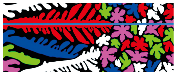
Fig. 8: Simulation results of dendrite morphology with V_c=1.2 \text{ K}\cdot\text{s}^{-1} and G=10 \text{ K}\cdot\text{mm}^{-1}
