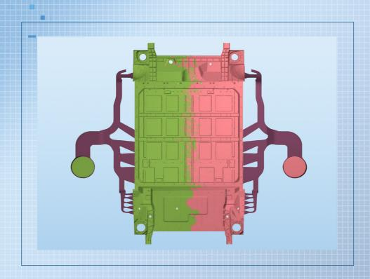
Simulation study on integrated bottom car body formation by high pressure die casting with a dual injection system
