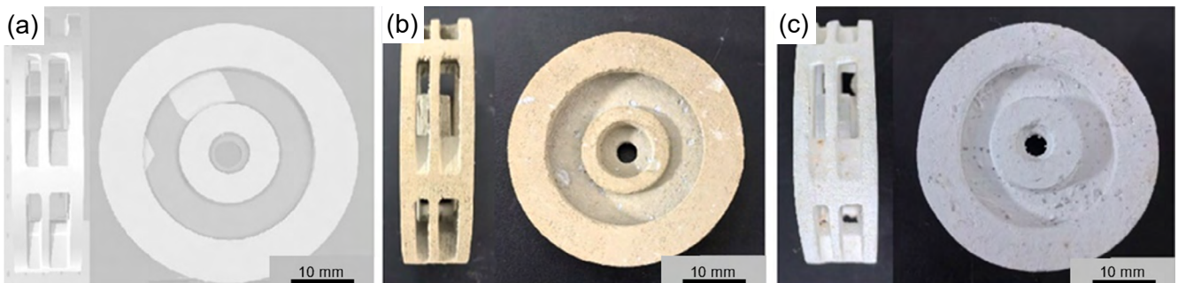
Fig. 14: Heavy calcium carbonate ceramic core of rotor part by binder jetting: (a) 3D model; (b) green body; (c) sintered part [70]
