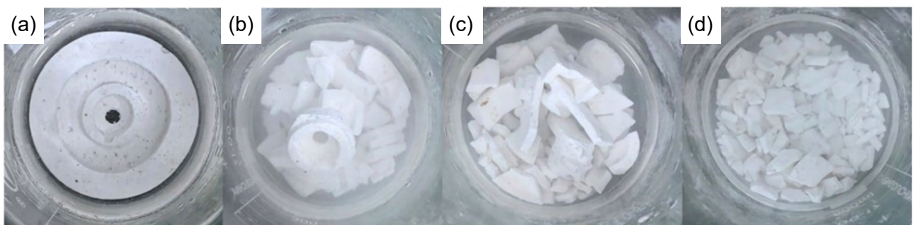
Fig. 15: Images showing the collapse effect of the ceramic core of rotors (a-d) [70]
