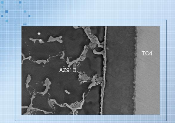
Effect of HEA/AI composite interlayer on microstructure and mechanical property of Ti/Mg bimetal composite by solid-liquid compound casting
