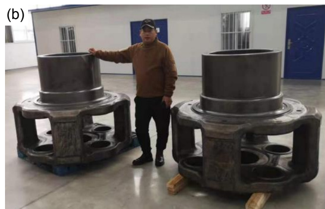
Fig. 10: ADI planetary carrier undergoing austenitization treatment at ADI treatments in Birmingham, UK (a) [16] , and ADI planetary carriers heat treated by Hubei ADI Material Tech Co., Ltd., Hubei Province, China (b)
