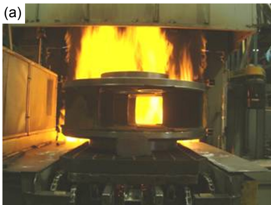
Fig. 10: ADI planetary carrier undergoing austenitization treatment at ADI treatments in Birmingham, UK (a) [16] , and ADI planetary carriers heat treated by Hubei ADI Material Tech Co., Ltd., Hubei Province, China (b)
