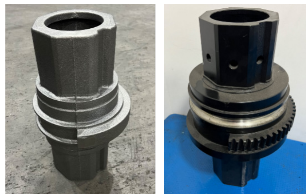
Fig. 8: Raw casting (left) and machined (right) ADI worm parts for solar PV trackers (courtesy Changjian Foundry)
