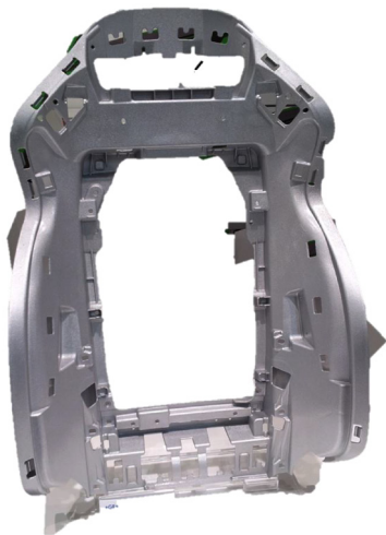
Fig. 7: Images showing Mg alloy seat frame applications in 2015 Mercedes-Benz SLK seat [24]
