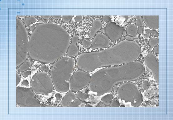
Effect of slow shot speed on externally solidified crystal, porosity and tensile property in a newly developed high-pressure die-cast Al-Si alloy
