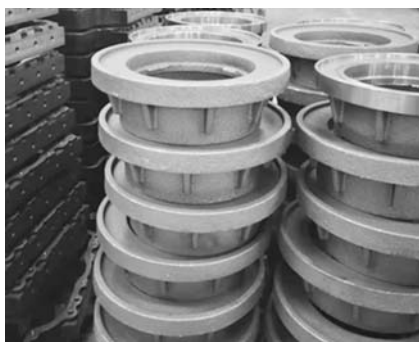
图4 钇基重稀土球化包芯线生产的球铁冲床配件 Fig. 4 Ductile iron punch accessories produced by the yttrium heavy rare earth spheroidized cored wire
