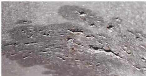
图5 冒口根部出现的缩松 Fig. 5 Shrinkage porosities appeared at the riser root
