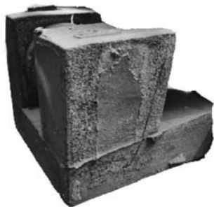
图12 加设外冷铁而孔不铸出的铸件轴承孔支撑架局部照片 Fig. 12 Photo of part of bearing platform of the casting with external chill settings but no hole cast out
