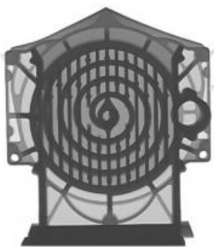
图15 铸件X射线检测结果 Fig. 15 X-ray detection result of casting
