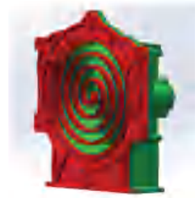
图2 铸件分型面设计 Fig. 2 Parting line design of the casting
