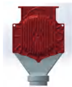
图3 铸件浇注系统设计 Fig. 3 Gating system design of the casting
