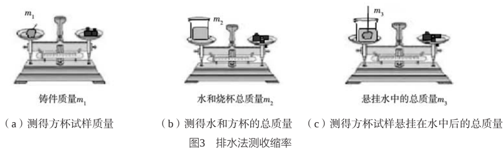
Fig. 3 Measuring of shrinkage rate by using of drainage method
