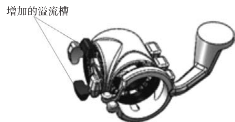
图10 优化方案三维图 Fig. 10 Three-dimension model of optimized die casting process
