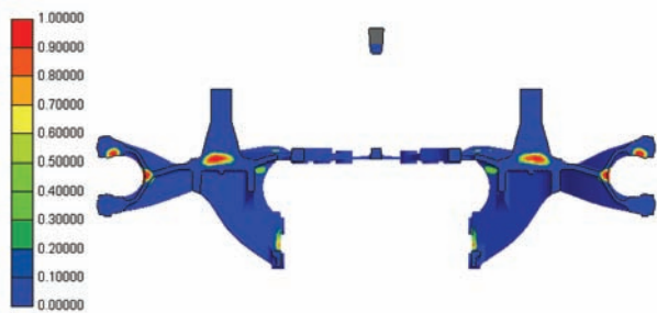
图6 铸件缺陷预测结果 Fig. 6 Prediction results of casting defects
