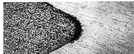
图3 铸锭与导向器叶片边缘接触处 Fig. 3 Contact area between the ingot and the guide
