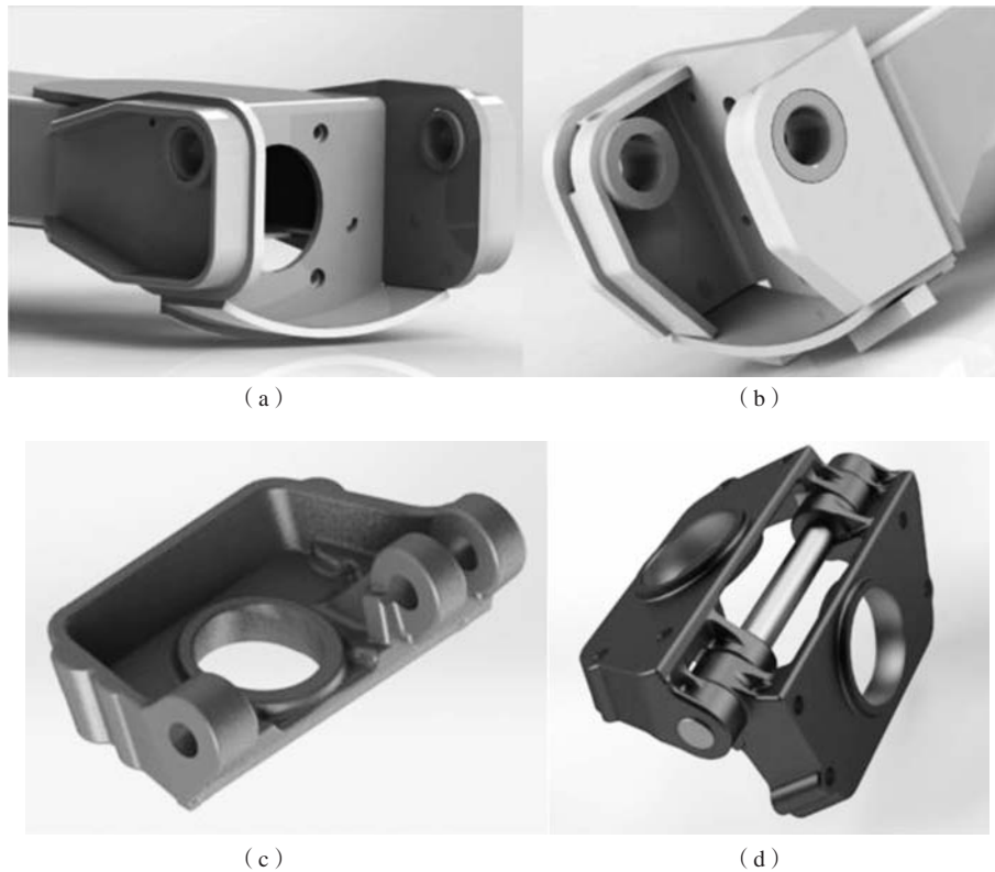
图5 原设计的两件式42个部件组装而成的泰德铰链 (a, b) 改为整体式一件ADI件 (c, d) Fig. 5 Original two-piece, 42-component assembled Tedder hinge (a, b) converted into a one-piece ADI casting (c, d)
