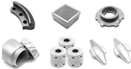
图7 升华三维钨合金打印样品 Fig. 7 Tungsten alloy printed sample
