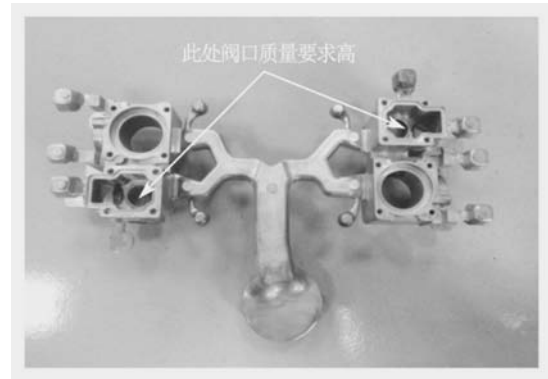
图9 阀体阀口表面质量要求高 Fig. 9 Valve body and port surface with high quality requirements
