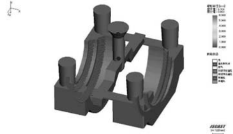
图3 铸造缺陷数值模拟 Fig. 3 Numerical simulation of casting defects
