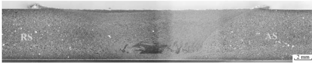
图3 ADC10合金搅拌摩擦加工横截面结构 Fig. 3 Cross-section structure of friction stir processing of the ADC10 alloy
