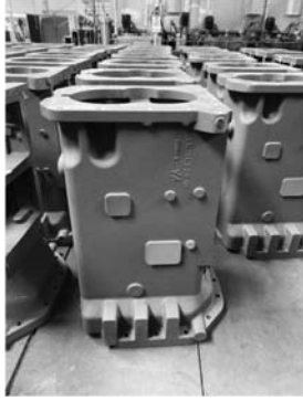
图17 铸件加工成品 Fig. 17 Finished castings
