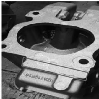
图4 本体取样位置 Fig. 4 Test sampling location of the cylinder head casting
