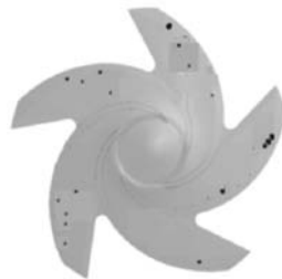
图9 工艺改进后缺陷模拟显示图 Fig. 9 The defect display of the casting after improved process
