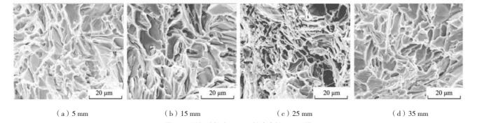
图9 不同振动幅度下A357铝合金的断口形貌 Fig. 9 Fracture morphology of A357 aluminum alloy at different vibration amplitude
