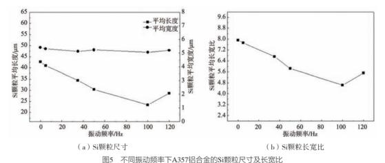
Fig. 5 Si particle size and aspect ratio of A357 aluminum alloy at different vibration frequencies
