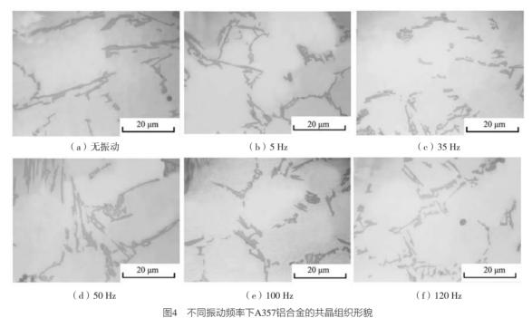
图4 个问题和颁唤下A337和口壶印光照组织形然 Fig. 4 Eutectic morphology of A357 aluminum alloy at different vibration frequencies
