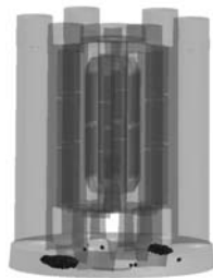
图4 低压浇注工艺疏松缺陷图 Fig. 4 Total shrinkage Porosity of the LPDC
