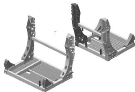
图14 铸件和型材焊后的总成件示意图 Fig. 14 Assembly diagram by welding of investment casting part and profiles
