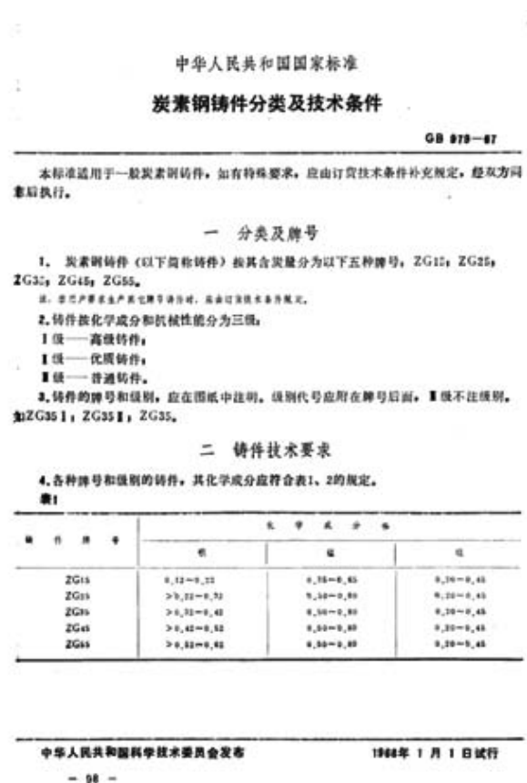
图3 GB 979—67《炭素钢铸件分类及技术条件》 Fig. 3 GB 979—67 Classification and technical conditions of carbon steel castings
