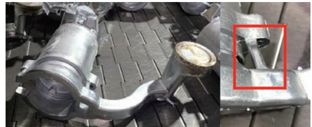
(a) 薄壁转向电机壳体铸件 (b) 辅助浇道
