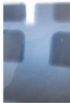
图13 铸件热节部位的X射线检验结果 Fig. 13 X-ray inspection results of the hot spot area of the casting
