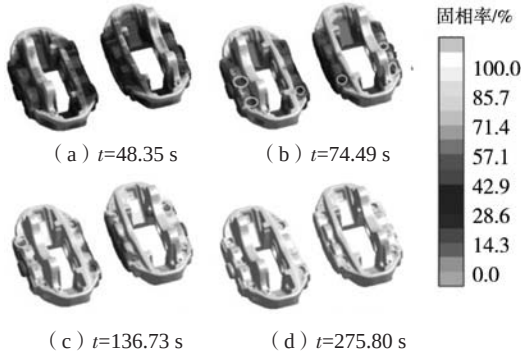
图2 铸件凝固过程中的固相率变化 Fig. 2 Changes of solid phase rate of the casting during the solidification process
