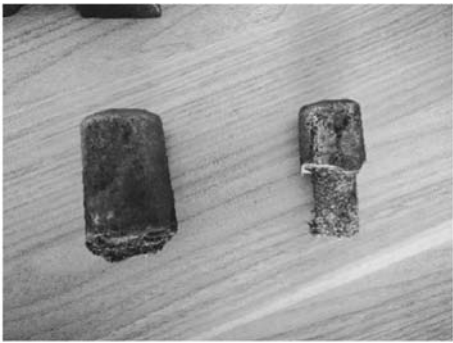
图8 设计更改前(左)后(右)冒口实物 Fig. 8 Riser pictures before (left) and after (right) design modification
